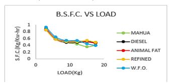
From the above figure we can see that BSFC decreases exponentially with load. Out of the fuel used, waste frying oil is found to have highest BSFC due to least energy content and diesel has the lowest BSFC.
