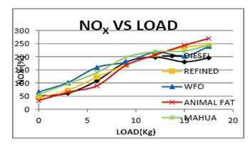
Figure shows the variation of *NOx* with load. *NOx* emissions of all biodiesel blends are higher than that of conventional diesel. The high combustion temperature and the presence of extra oxygen are the main parameters for more *NOx* emissions. This can be reduced with proper adjustment of injection timing and recirculating the small portion of exhaust gas with fresh air during the induction process.
