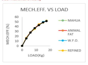
The difference between indicated powers is the indication of power loss due to friction in mechanical components of the engine which form the basis of mechanical efficiency. The high value of viscosity may lead to some problem in pumping and atomization in the injection system of the diesel engine which reduces mechanical efficiency of biodiesels.
