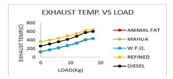
Biodiesel has higher exhaust temperature than diesel because of high loads .This is due to the fact that biodiesel includes constituents having higher boiling point than diesel. Thus the constituents were
