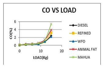
Fig. shows the variation of co with respect to load. It is learned that the variation in *CO* emissions for all biodiesel blends and diesel is fairly small. This may be due to the oxygen content and less *C/H* ratio of biodiesel that causes complete combustion. However, it is revealed that the decreasing trend of *CO* emission does not rely on biodiesel percentage in the blends
