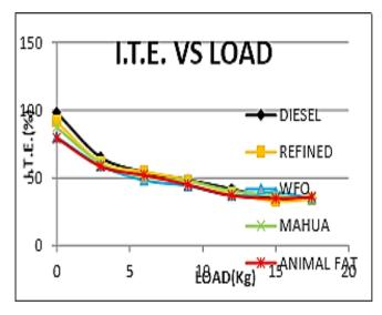
Out of the biodiesel produced Soya bean gives the indicated thermal efficiency very close to the diesel. As the source soya bean oil was quite fresh and similarly waste cooking oil gives the least thermal efficiency due to overheating.
