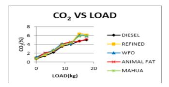
The above figure shows the variation of percentage of *CO2* vs load. It is clearly seen from the figure that with the addition of biodiesel with the diesel engine causes higher amount of carbon dioxide at tail pipe. For most of the load waste frying oil has highest percentage of co2 emission due to highest oxygen content.
