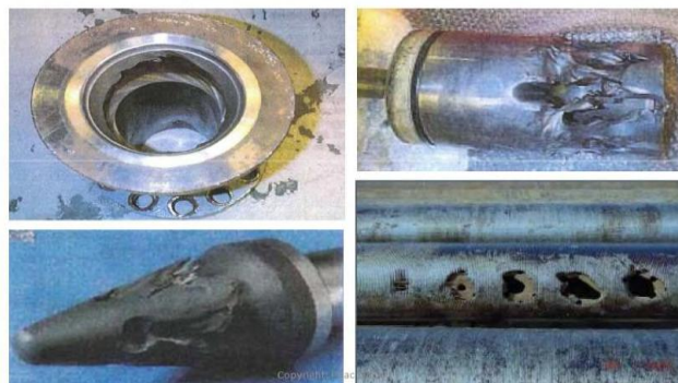
Figure – 3: The consequences of formation sand production, Source: Sanjay K. Dhiraj Dy. SRE, G&R Deptt.
