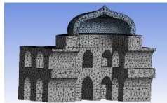
Fig. (4) Finite element meshing of Khusrobagh Tomb with 71839 of SOLID 187 elements and 8615 of SURF154 elements.
