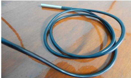
Figure 5. The DS18B20 temperature sensor used in the RWTMS
